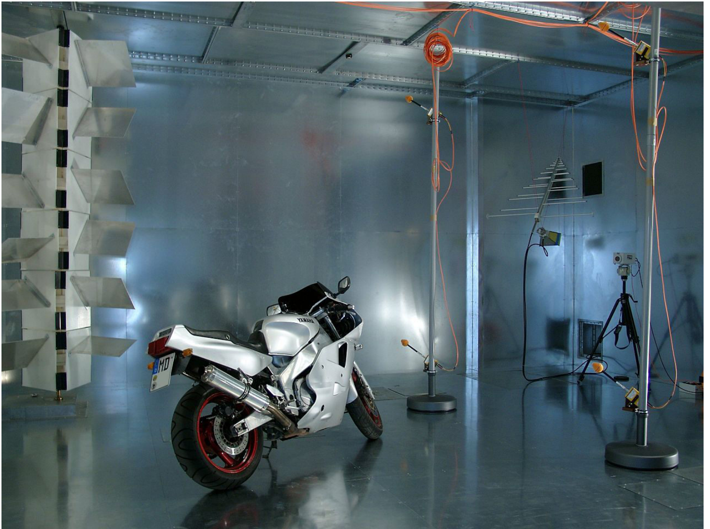
A motorbike undergoes testing in a reverberation chamber - © Dr. Hans Georg Krauthäuser [CC BY-SA 3.0] via Wikimedia Commons
