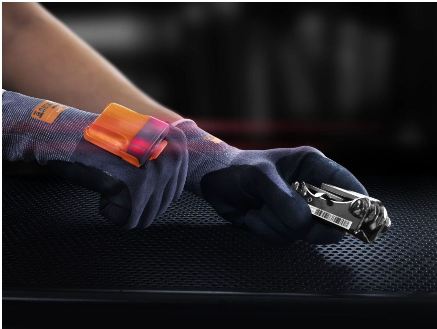
The ProGlove recognises whether the user is holding the right component or product - Source: ProGlove
