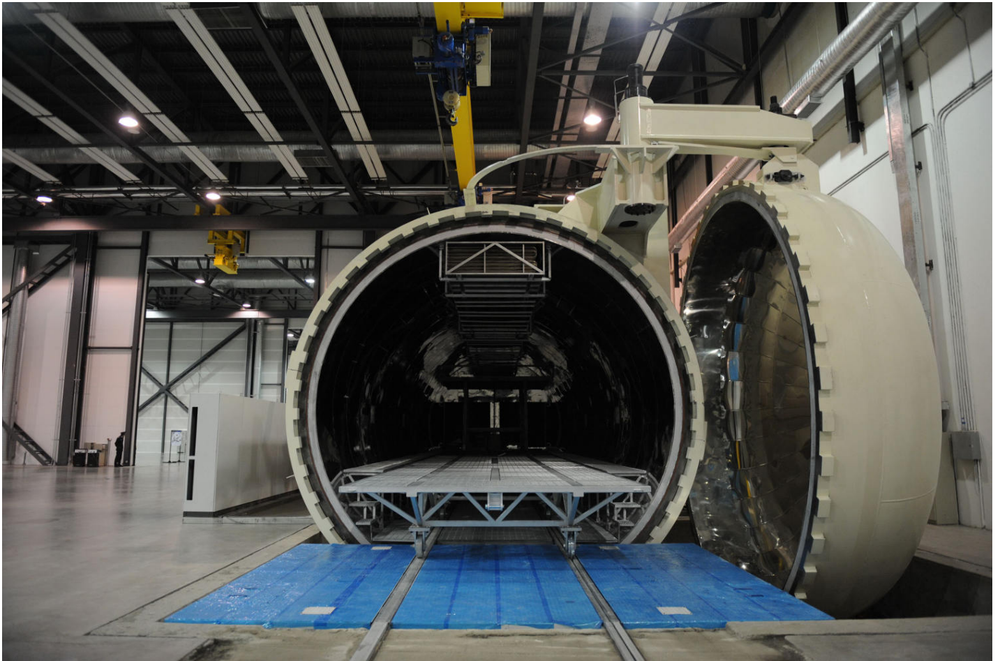
Airbus's he enormous Harbin Hafei autoclave produces composite materials for the A350 XWB - © Airbus SAS 2017
